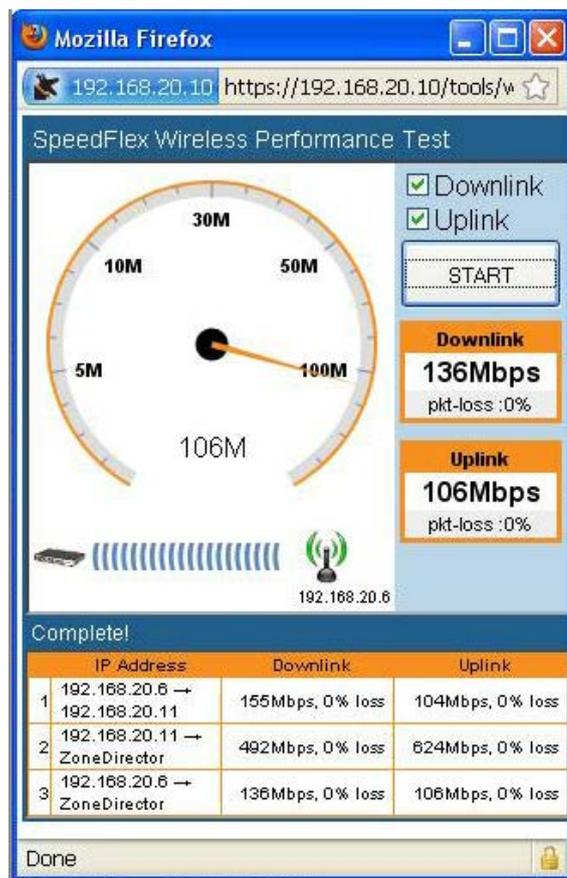
SpeedFlex® is a unique wireless performance test tool integrated within the ZoneFlex® family of centralized controllers that measures the Wi-Fi throughput of associated wireless LAN clients.
